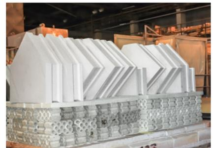
Components on a tunnel kiln car after firing
