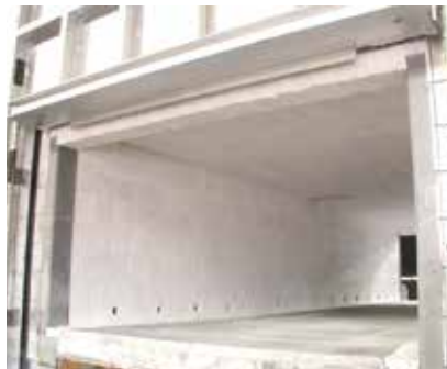
HTW lining for bogie-type furnaces
