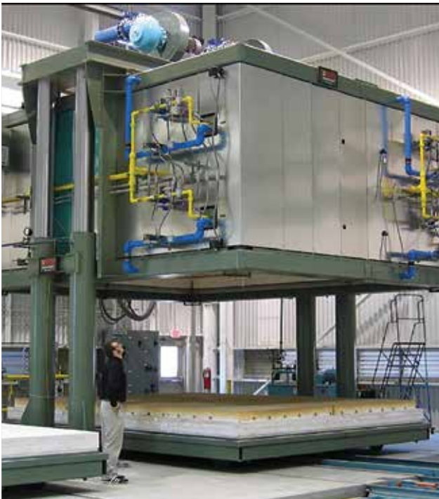
Bell-type furnace with HTW modules
