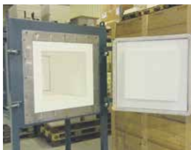
ACS roof for HT furnace
