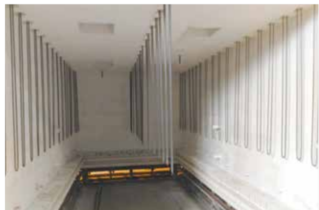
Electrically heated bogie hearth furnace with lining made of Altra modules for application temperature of up to 1600 °C
