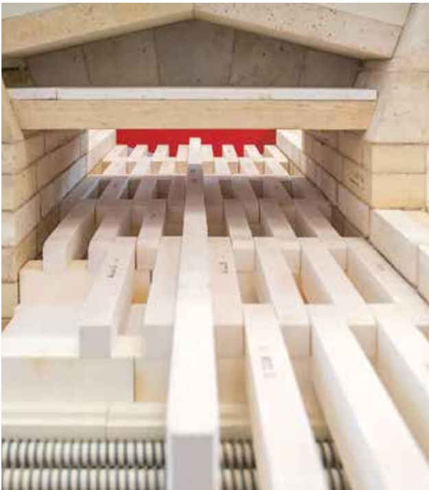
Pusher plate furnace
