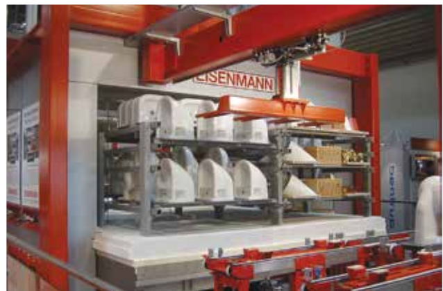
Tunnel furnace for the firing of sanitary ceramics and clinker
