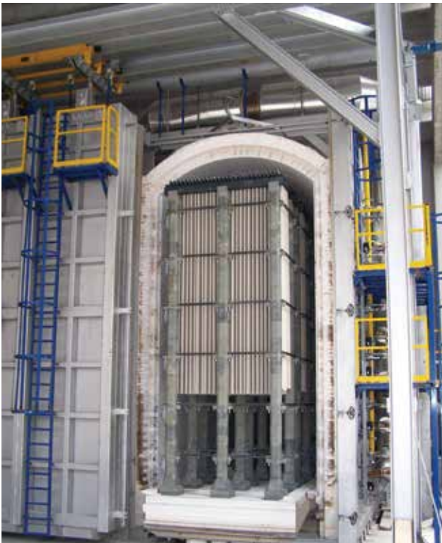
Bogie hearth furnace for the firing of ceramic pipes Height: 8 m; width: 4 m; temperature: 1650 °C
