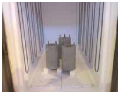
HT furnace up to 1700 °C with ACS components in roof and wall
