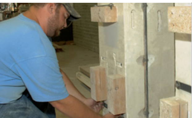
Removal of a refractory furnace liner from the mold.
