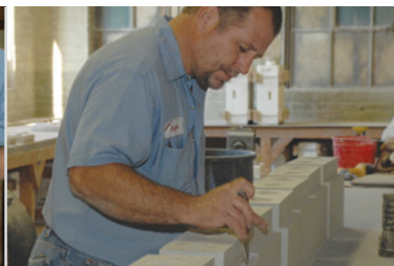
Finish work on green burner blocks prior to entering the drying room.
