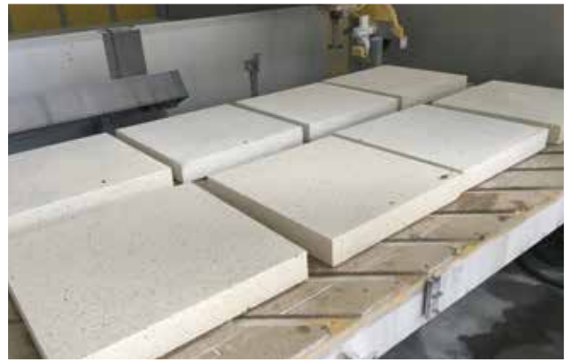
Bottom sub-paving blocks after machine grinding
