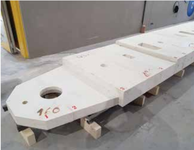
Pre-assembled forehearth and spout cover blocks
