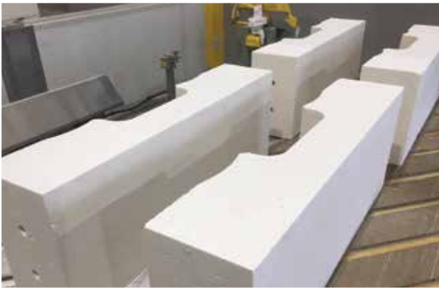
Forehearth cover blocks under machining
