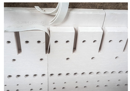
CNC-milled sidewall elements with numerous feedthroughs
