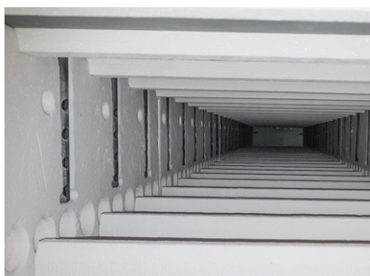
View into the furnace in throughput direction, with blowing-in and exhaust systems on the left and right
