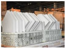
Components on a tunnel kiln car after firing
